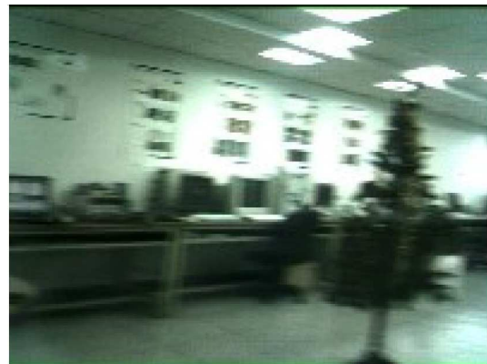
Fig. 1. Illustration of the rolling shutter effect. The Christmas tree and the vertical edges of the scene appear slanted as the camera pans across the scene.
